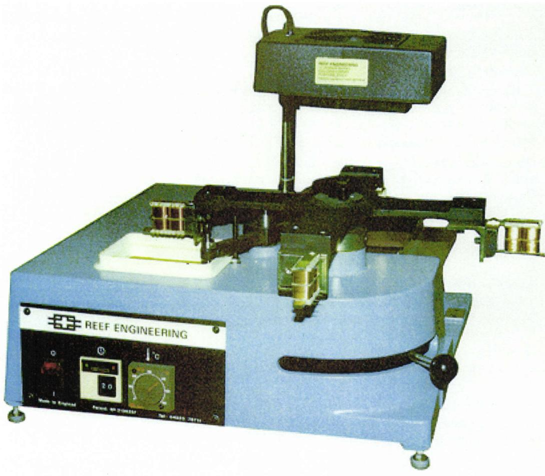
The OTTER soldering machine has been specifically designed to meet the requirements of the smaller winding shop, and with its realistic price, brings the advantages of machine soldering within easy reach of all coilwinding companies. Interchangeable turret assemblies enable small batch runs of coils to be soldered quickly and economically, with a consistent quality that cannot be matched by hand dipping.
